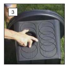
Check to make sure you have completely tightened the nut and that the seal is not loose on the D-Box.
