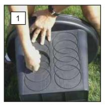
Lubricate your blade and cut following the angle of the circle impressions.
